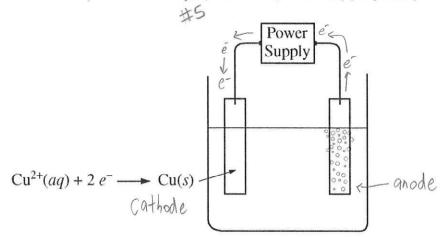
3. An external direct-current power supply is connected to two platinum electrodes immersed in a beaker containing 1.0 M CuSO<sub>4</sub>(aq) at 25°C, as shown in the diagram above. As the cell operates, copper metal is deposited onto one electrode and O2(g) is produced at the other electrode. The two reduction half-reactions for the overall reaction that occurs in the cell are shown in the table below.
