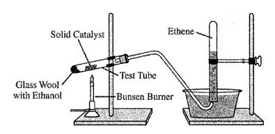
4. Ethene,  $C_2H_4(g)$  (molar mass 28.1 g/mol), may be prepared by the dehydration of ethanol,  $C_2H_5OH(g)$  (molar mass 46.1 g/mol), using a solid catalyst. A setup for the lab synthesis is shown in the diagram above. The equation for the dehydration reaction is given below.
