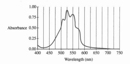
(a) To determine the optimum wavelength for an experiment that measures the concentration of  $MnO_4^-(aq)$ , the student takes a sample of the solution and measures the amount of light absorbed by the sample over a range of wavelengths. The data are plotted in the graph shown. Identify the optimum wavelength that the student should use for the experimental procedure.
