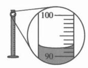
(i) The student uses a 100.0 mL graduated cylinder to measure a certain volume of  $KMnO_4(aq)$  stock solution, as shown in the diagram given. What volume should the student record?
