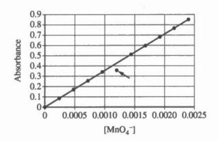
(c) Assuming that all lab equipment is functioning properly, identify which one of the procedural steps the student could have executed incorrectly that would explain why the marked data point is below the line of best fit.
